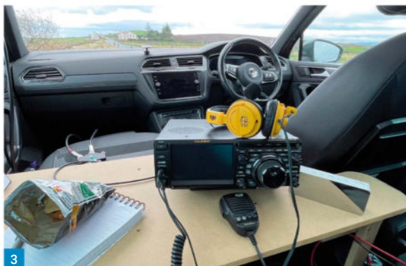
Fig. 3: Max Townsend G4SDX's Yaesu FTdx10 incorporates the 70MHz band.
