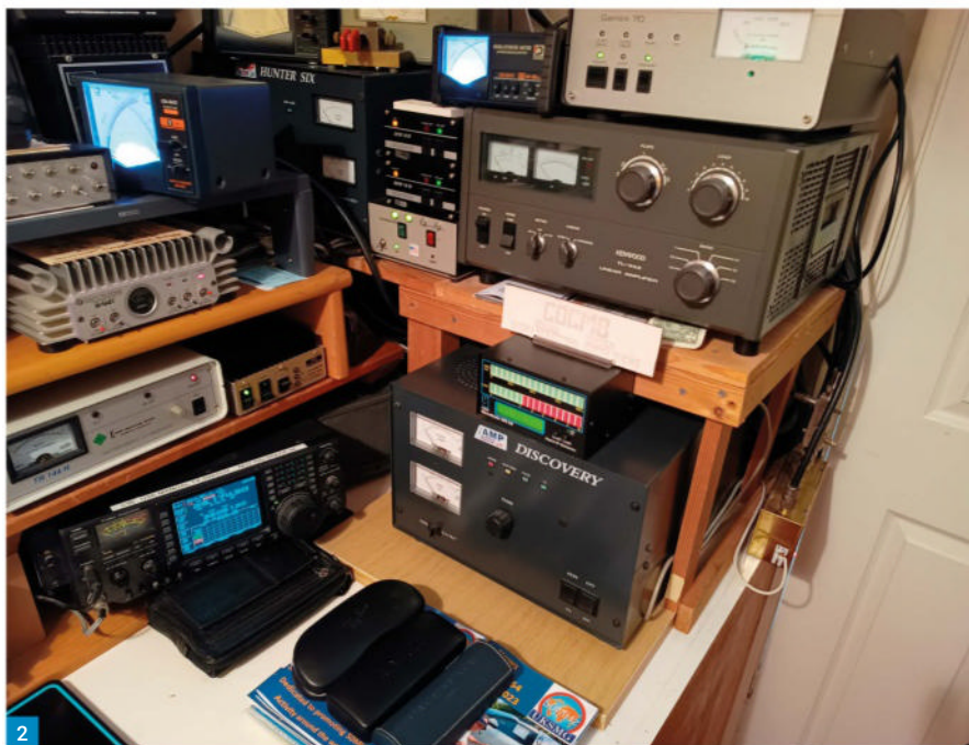
Fig. 2: More shack equipment: on the right is a Kenwood TS-22 HF band linear and, below, a Linear Amp 'Discovery'. Fig. 3: Principal rotary antennas mounted on telescopic mast: dipole for 10m/15m/20m; 15-element 70cm beam; 5-element 6m beam; F9FT 'Tonna' 17-element 2m beam. Fig. 4: 3-element 4m rotary Yagi. The pole on the carries supports a doublet that zig-zags around the garden.
