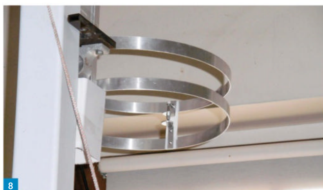
Fig. 6: Details of the indoor feedpoint adjustment. Because it is indoors, I have not got around to making it permanent. The capacitors are small airspaced of 0.5-3pF. I have found 2/3mm diameter bolt set in a captured nut to be a good practical method when opposed by a small plate a few millimeters away, as illustrated in Fig. 8. Fig. 7: MMANA (method of moments) model of a skeleton slot and the resultant far field radiation. Omnidirectional in azimuth, vertically polarised. The elevation angle depends on the height above ground. Four illustrations: 14MHz at 1.5m height on a fence (25° elevation lobe), 29MHz at 6m above ground (10°), 50MHz 6m above ground where the main first lobe is \sim 1.5^\circ elevation angle, 145MHz 1.2° elevation angle both corresponding to my loft mounting place above ground. Fig. 8: Details of the tuning capacitor. I found a 2/3mm, self-captive screw and an opposing plate is adequate. My calculations indicated bigger plates but not with the antenna dimensions given in Table 1. This helps simplify the capacitor arrangement.
